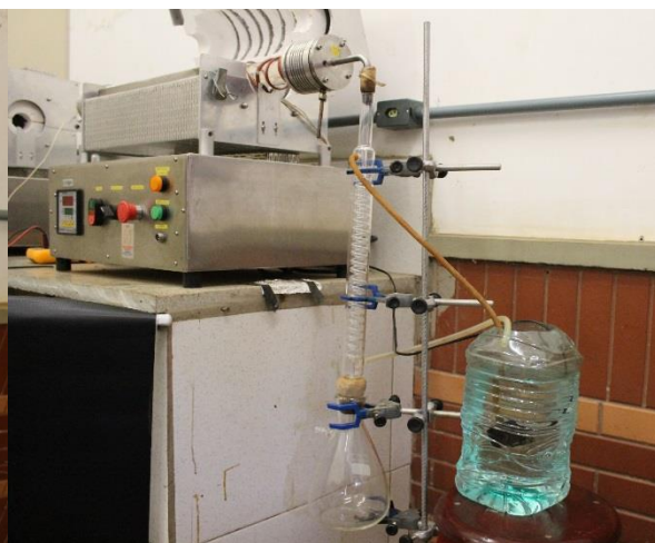
Figure 9 - Condensation system implemented in the fixed bed chemical reactor.
