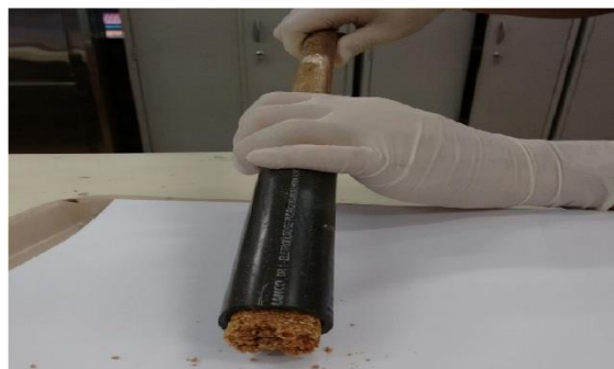
Figure 7 - Production of handmade briquette.
