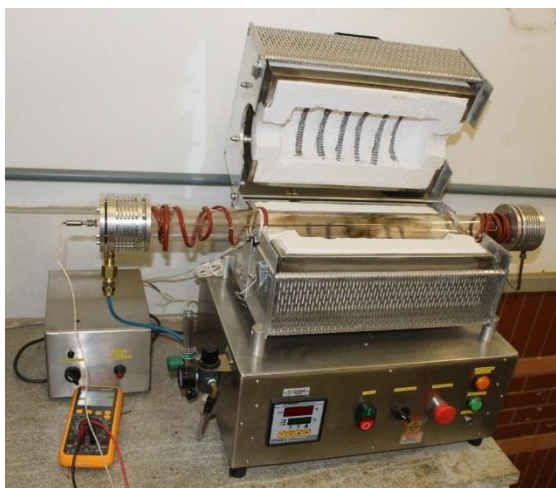
Figure 8 – Bipartite Fixed Bed Reactor.
